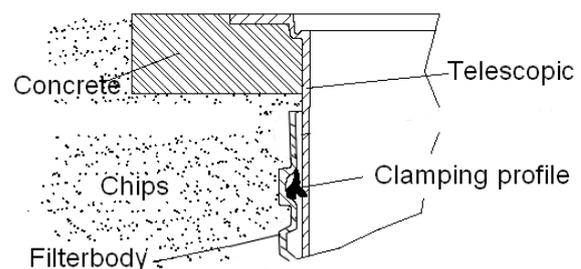
with the lubricating soap included in the delivery (use no lubrication that is mineral oil based). **Attention:** If the lubricating soap becomes dry and the telescope becomes difficult to move then there is the danger that the sealing ring will be forced out of its recess. Before filling the sealing ring must be checked once again that it is seated correctly in position. The telescope must be sufficiently embedded and supported that no forces are transferred to the housing.
