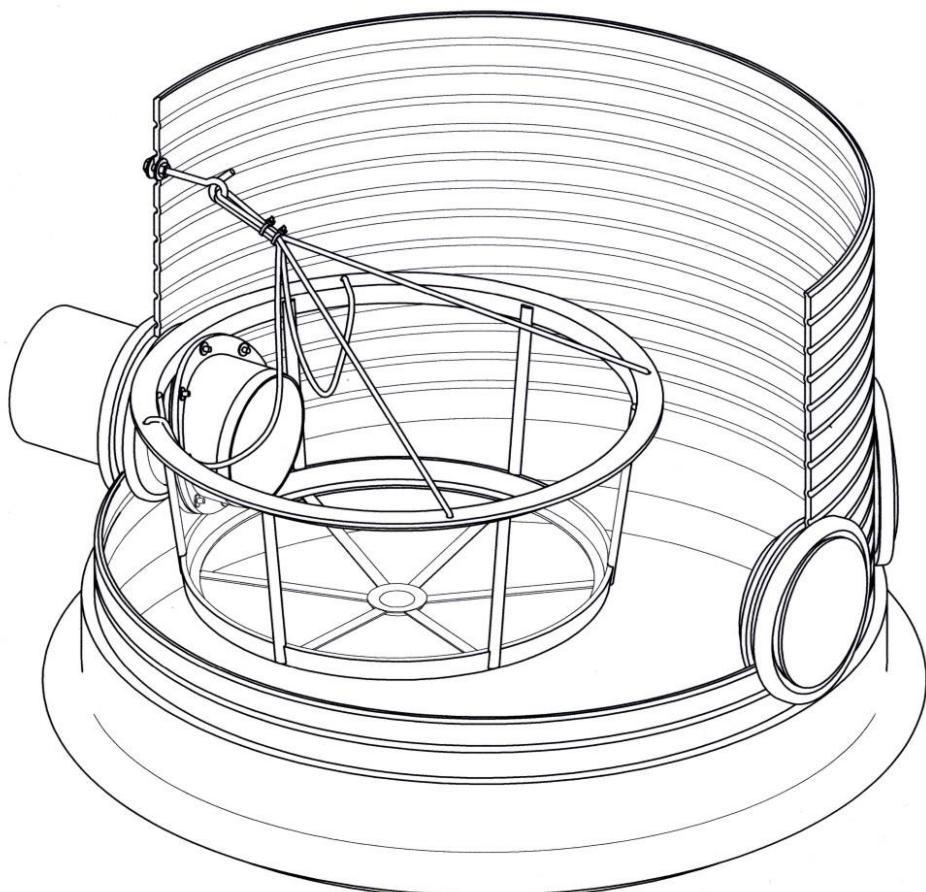
Design example using parts in the scope of delivery: a filter basket, pluggable, a screw hook, two ropes, two cable straps
