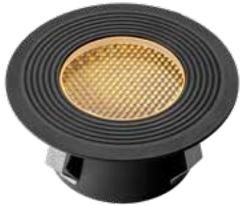
Onyx 90 RA (245D) Aluminium - Anthrazit LED 2 W 2.700 K 76 lm 78 x 105 mm (H x Ø) Bohrung 90 mm € 75,00
