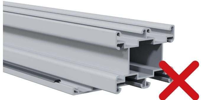
It should be noted that the seals used contract after installation in the profile channel. We recommend fitting the seals on both sides with an excess length of at least 25 mm and cutting them flush with the profile channel after the sealing have settled. In the case of seals with special lengths, we point this out in the installation instructions. Denominations are possible for the seals.
