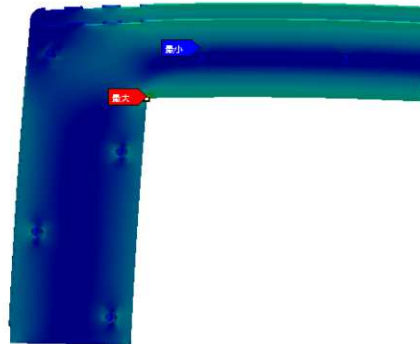
Figure 4-8 Diagram of equivalent plastic strain (0.0024)
