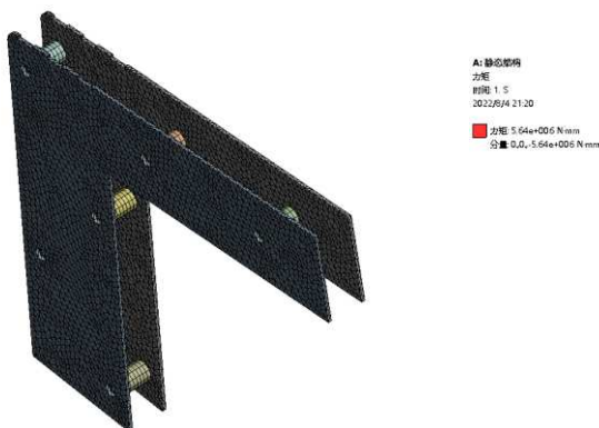
Figure 4-2 Diagram of corner piece finite element model
