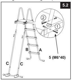
**IMPORTANT:** One side at a time. Do not attach the other side of the ladder until the U-shaped top rail is installed. Make sure all nuts and bolts are securely tightened. Do not fully tighten fasterners until last assembly operation.
