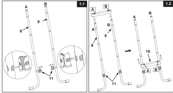
**IMPORTANT:** Ensure the J-shaped legs are pointing outwards before installing the steps.
