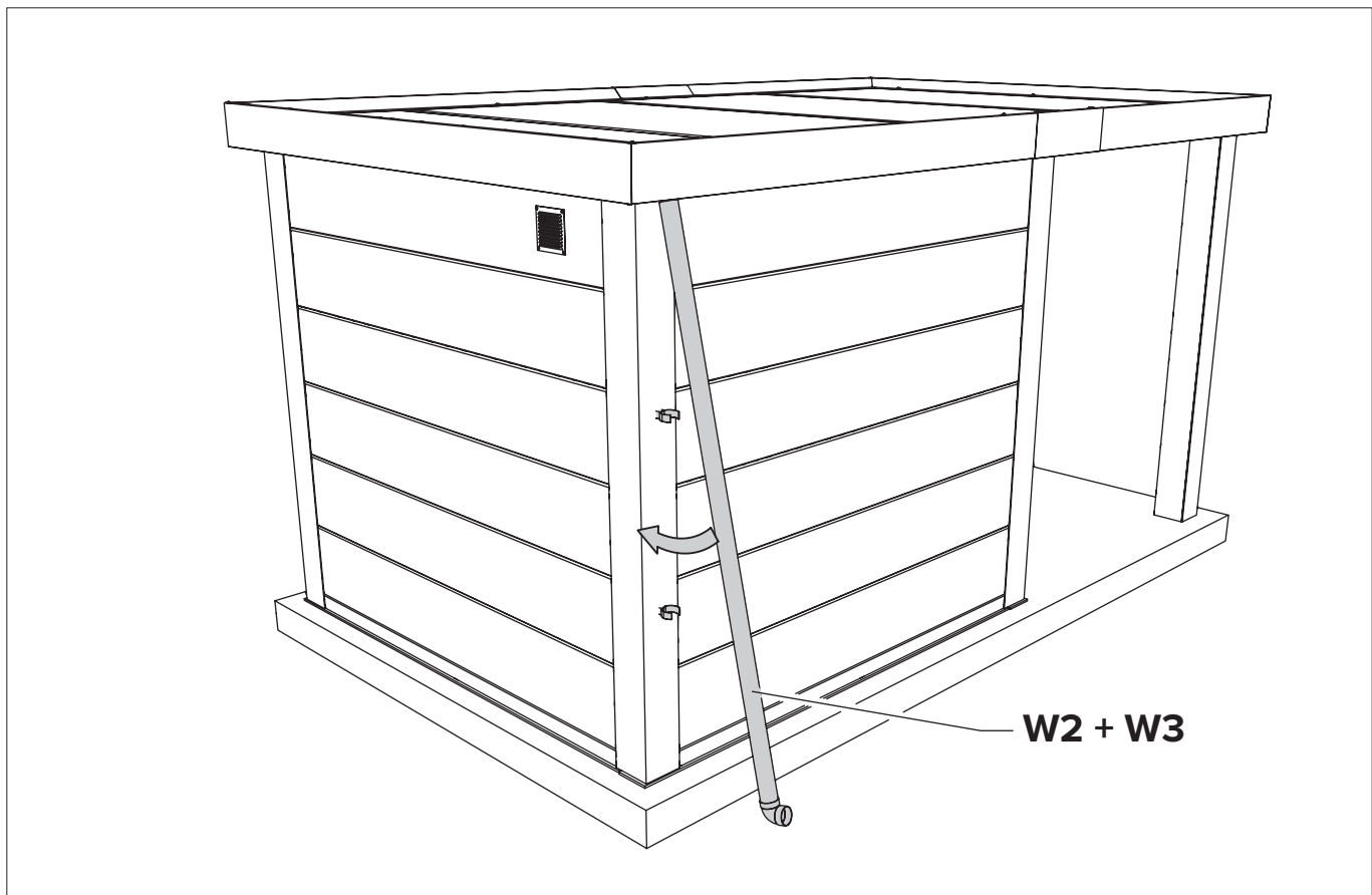
Drain / Afwatering / Drainage / Drainage
